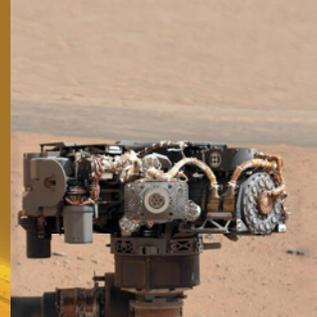
The Alpha Particle X-Ray Spectrometer (APXS) on Curiosity with the Martian landscape in the background. IMAGE COURTESY OF NASA/JPL-CALTECH/MSSS
