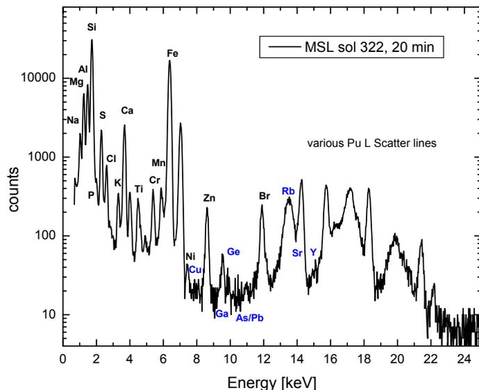
**FIGURE 1** X-ray spectrum of the rock Ailik measured in Gale Crater on sol 322 over a 20-minute period. Plotted is the logarithm of the X-ray counts versus X-ray energy (in thousands of electron volts). The peaks labeled in black are for the 16 standard elements. The blue labels indicate elements quantifiable when in elevated abundance. The analysis procedure transforms the peak areas into concentrations of the respective element oxides.
