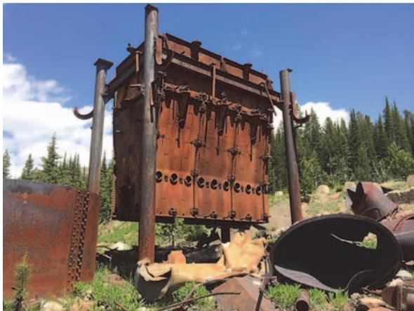
**FIGURE 1** This abandoned early 1900s copper blast furnace in the New World Mining District (Montana, USA) is symbolic of the full thermodynamic cycle: energy was once inputted to liberate Cu from its native minerals, whereas the iron furnace itself is now corroding back to its native oxides. PHOTO COURTESY OF EDWARD MEYER (DARTMOUTH COLLEGE, USA).
