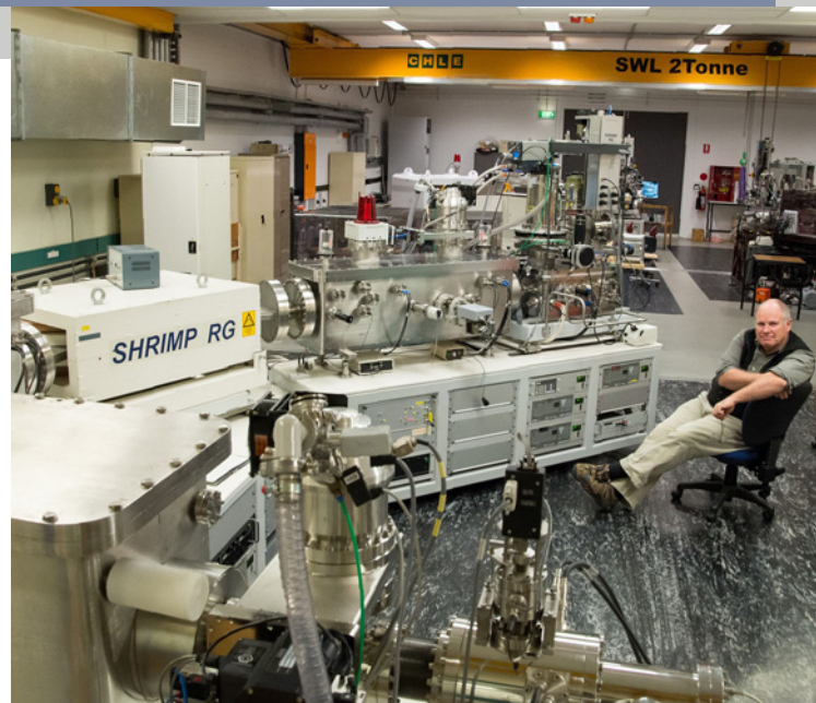
FIGURE 1 The sensitive high-resolution ion microprobe (SHRIMP) lab at the Australian National University houses three different ion microprobes, with plenty of surrounding space for modifications and installation. Prof. Trevor Ireland for scale.
