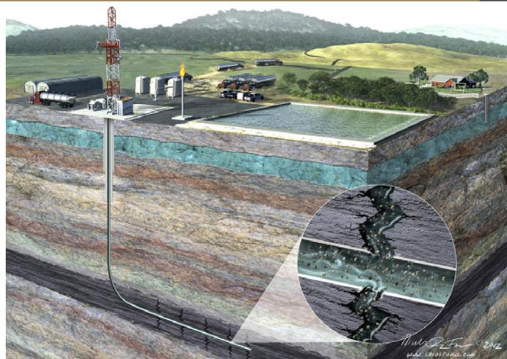
**FIGURE 1** Artist's rendering of a horizontal well drilled for shale gas production (COURTESY N. FULLER, SAYOSTUDIO.COM). Typically, the vertical section of the well is drilled, cased, and cemented to a depth of 2–3 km and then the well is drilled horizontally through the shale for about 1.5 km.
