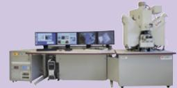
Quantitative microanalysis & X-ray mapping at sub-micron spatial resolution. Benchmark detection limits for trace and minor elements.
