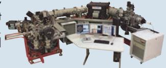
**NanoSIMS 50L** ion microprobe for high sensitivity, high lateral resolution analyses.
