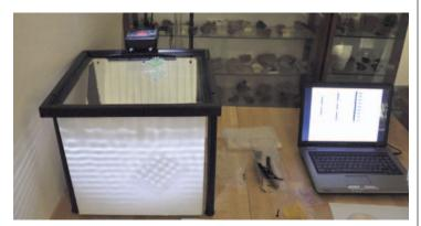
A ripple generator with a strobe light source used to show different kinds of wave patterns and their interactions
